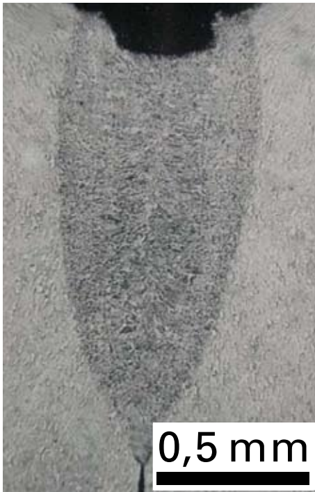
Laser weld in steel (3 kW at 9 m/min)
