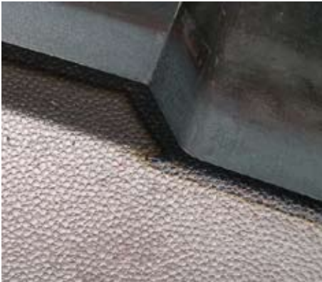
Laser hardened sealing edge of a plastic injection mould
