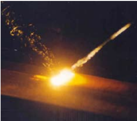
Laser melting of cast iron
