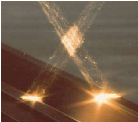
Laser hardening a folding tool using double beam optics
